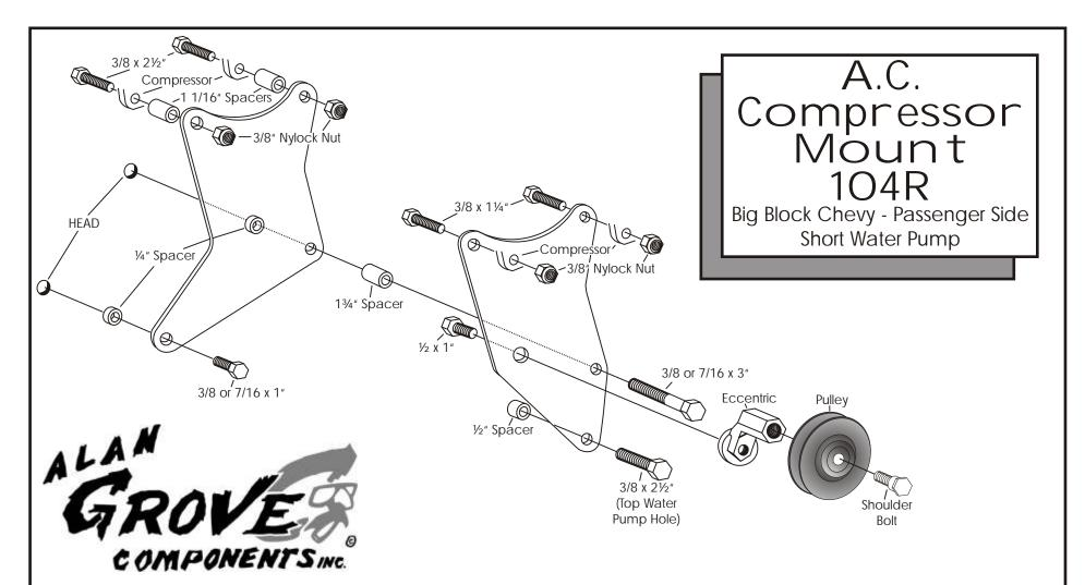
NOTE: Some heads have 3/8" bolt holes and some have 7/16". This kit includes both sizes of bolts for these holes.
