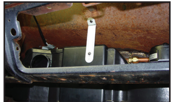
Photo 5 - Install Unit Support Bracket
