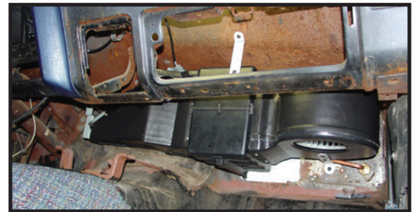
Photo 4 - Install Unit to Firewall
