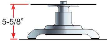
Short water pumps were used on engines for passenger cars thru 1968 and trucks thru 1972.
