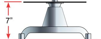
Long water pump were used on engines for passenger cars 1969 & up and trucks 1973 & up.
