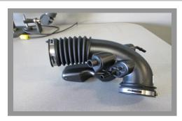
Loosen the (2) clamps on the air inlet tube at the air box and throttle body. And remove the air tube from the vehicle.
