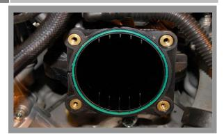
Wipe off the stock rubber throttle body gasket to remove any oil or debris. You will be reusing this gasket. Connect the motor plug to the BBK Throttle Body and install it onto the intake manifold. Use the supplied bolts to secure the throttle body to the intake manifold.
