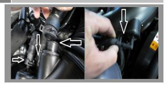
• Disconnect the sound tube and the (3) smaller plastic breather hoses from the air inlet tube.
