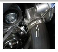
Loosen the clamp on the air inlet tube that connects to the throttle body using a flat head screwdriver or 7mm socket. Remove the air inlet hose by pulling it towards the front of the vehicle and slightly wiggling it side to side.
