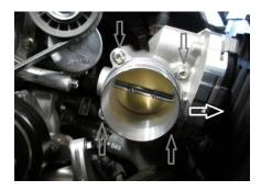
Unplug the wiring harness on the side of the throttle body that is located between the throttle body and air box. Remove the (4) 8mm bolts that hold the throttle body to the intake manifold and remove the throttle body from the vehicle.
