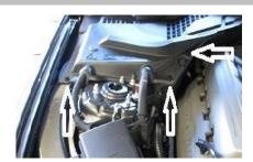
Remove the (3) screw pins that hold the battery cover to the body lift up the battery cover and disconnect the negative battery terminal using a 10mm socket.
