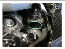
Be sure to clean the O-Ring of any oils or dirt before installing the BBK throttle body.
