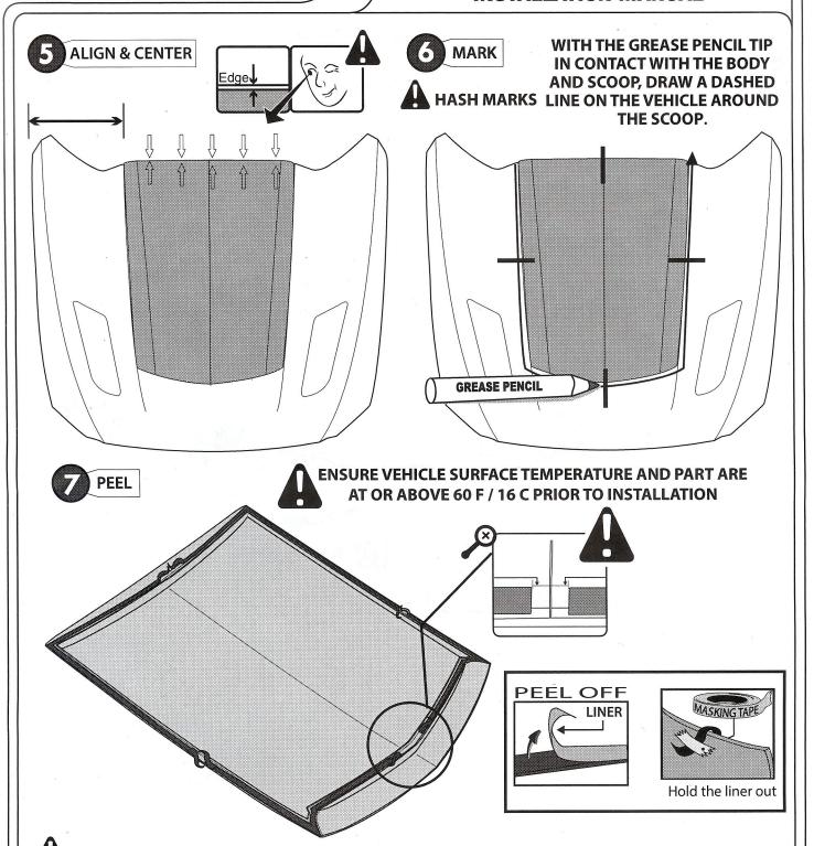
A full surface contact between tape and substrate is important for good adhesion performance.
