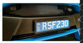
**Note:** The mounting base and bracket can be installed off centre by following the same directions, just not centering it. Additionally, the bracket angle can be adjusted. It is set at 80° up. If you need to adjust the angle to 90° or whatever angle you desire, simply place the slotted portion of the bracket into a bench vice and set your angle.
