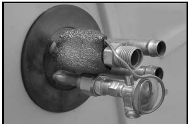
PHOTO #5 (Shown with Expansion Valve)
