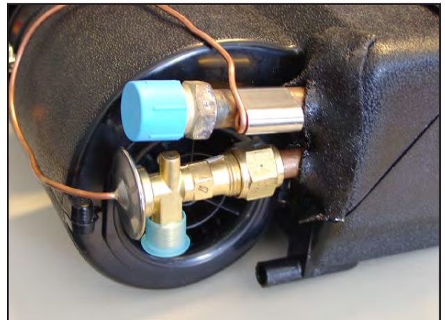
Photo 1 - Install Expansion Valve
