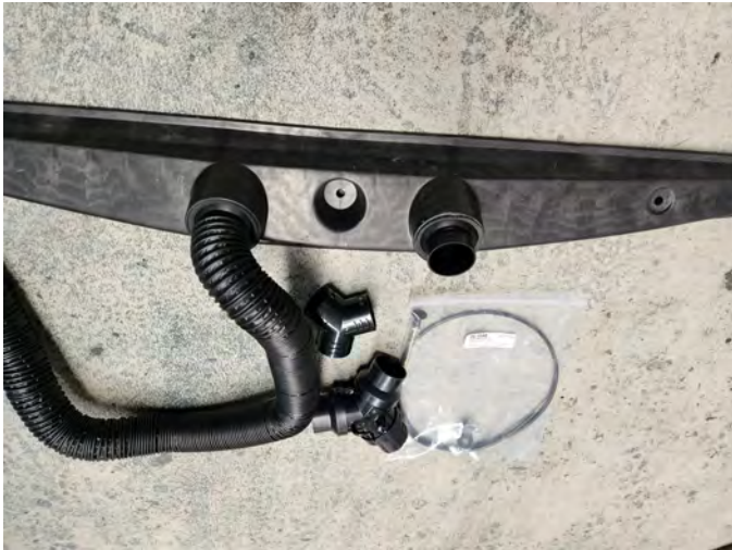
Photo 7 32-16A adaptors to defrost chamber
