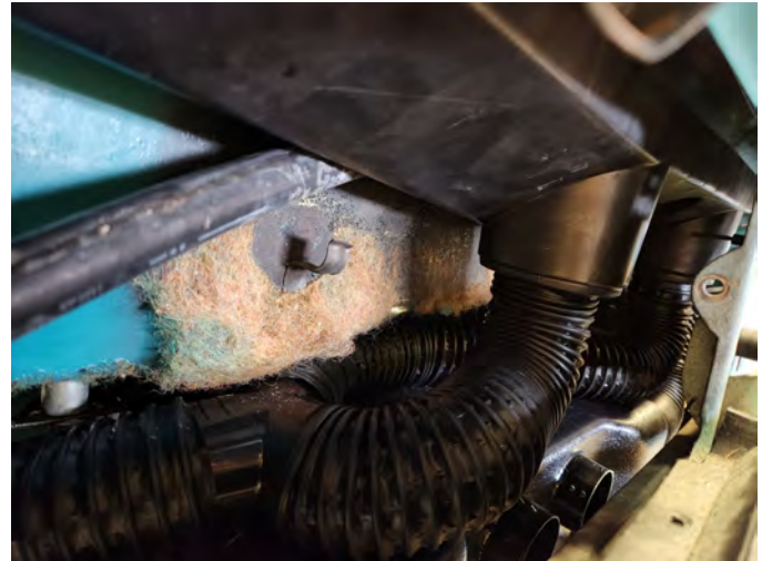
Photo 8 - 32-32 Y piece to defrost chamber
