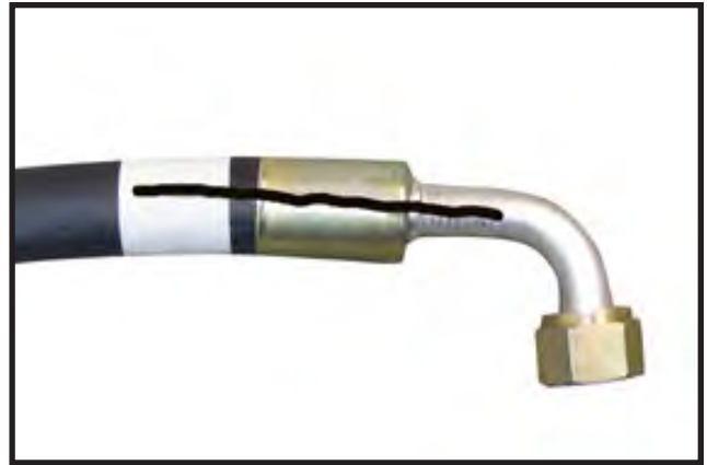
Photo 9 - Mark Position of Fittings on Hose
