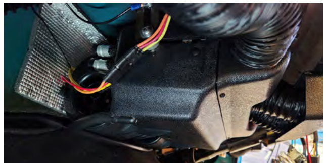
Photo 4 - Mount Evaporator to Dash
