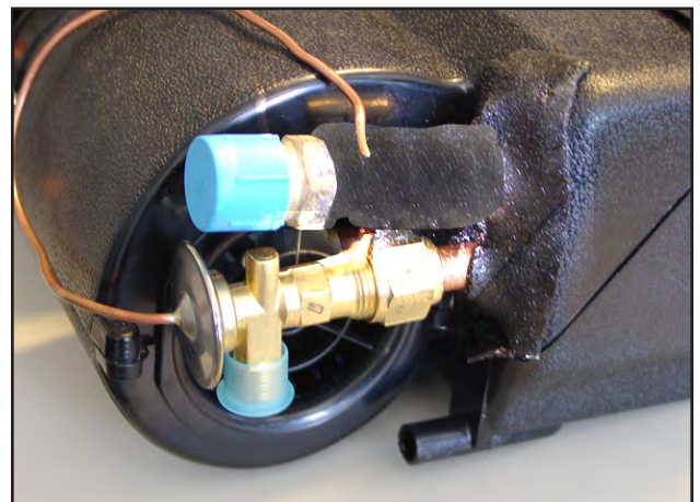
Photo 2 - Wrap Sensor With Insulating Tape
