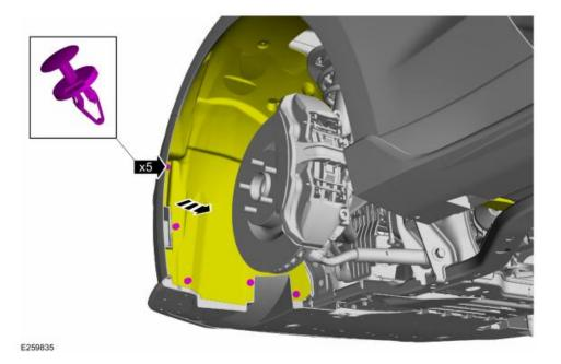
3. Remove the push pins, screws and the lower air deflector. Torque: 18 lb.in (2 Nm)
