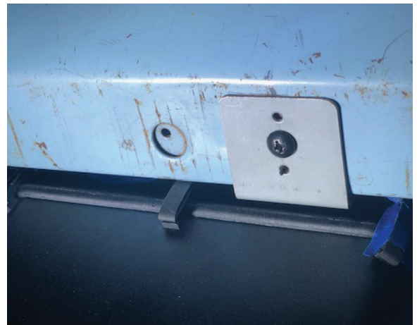
Photo 5 - Attach front bracket to dash
