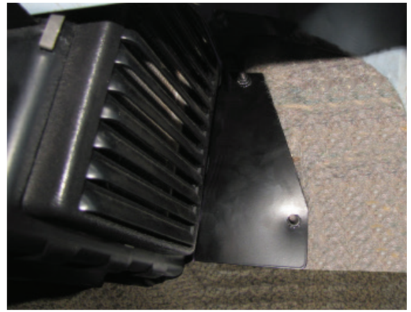
Photo 3 - Install unit to fire wall.
