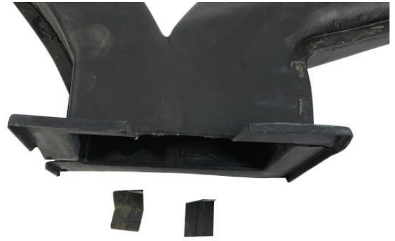
Photo 6 - Remove Tabs from defrost duct
