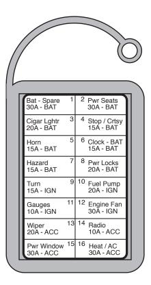
Fuse label on inside of Fuse Block cover
