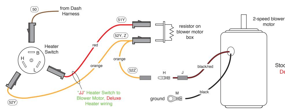
Figure "F" Stock Heater Switch and **Deluxe** Blower Motor connections
